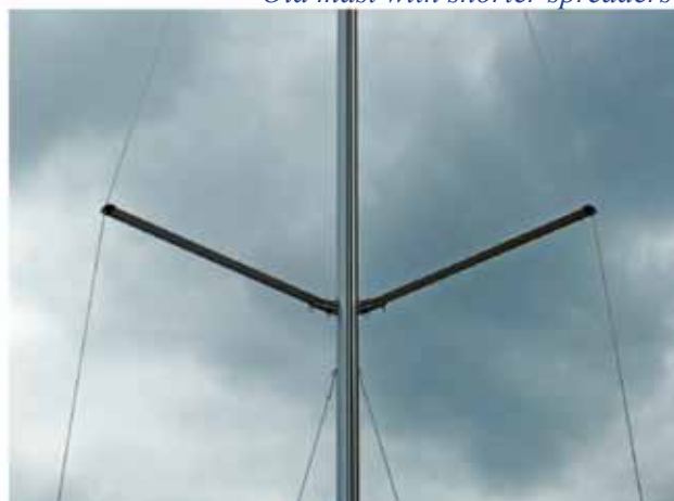
New mast and spreaders give a different shroud angle
